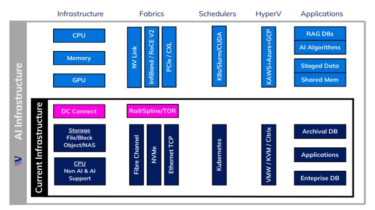
Current infrastructure environments are typically made up of the components in the black box. Al infrastructure environments include all those and the more specialized components for advanced AI workloads.
